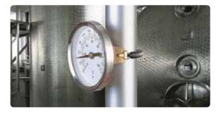
This easy to use surface pipe thermometer features a  $\emptyset60$  mm stainless steel dial and indicates temperature over the range of 0 to 120 °C or 32 to 250 °F. The  $\emptyset50$  mm dial face has a clear, graduated scale indicating temperature in 2 °C and 4 °F divisions.
