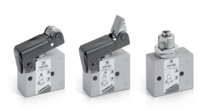
The mechanically operated Series 2 miniature valves with 3/2 normally closed function are available with M5 threaded ports or with an integrated super-rapid fitting for dia. 4 tubes. The devices are actuated by a plunger, roller/lever or a unidirectional lever.
