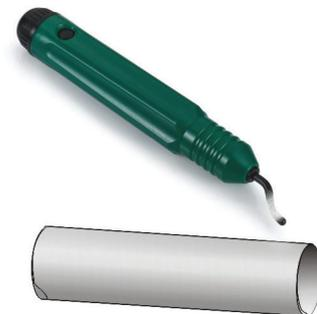
Deburr and remove any swarf with a deburring tool (209 0042 00) and a file for diameter between DN63 to DN200.
