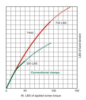
"TriTorque" clamps deliver almost three times the torque rating of conventional clamps.
